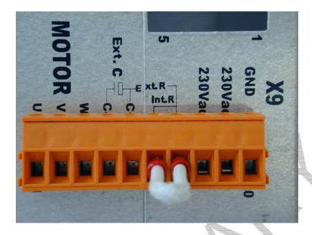
The XtrapulsPac drive is equipped with an internal 100  $\Omega$  / 35 W braking resistor. Its connection is made by means of a wiring bridge between pins 6 and 7 of the X9 connector. If the required rated power of the braking resistor is higher than 35 W or if the pulse power is higher than 1500 W, a larger external dp 50/200 power resistor must be mounted.
